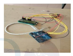
Figure 1: Arduino with LCD interfacing
