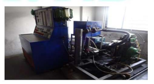
Fig: 2 shows EGR set to the Single cylinder Diesel Engine
