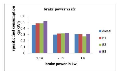
5.2 Brake power on X-axis and Specific Fuel Consumption on Y-axis
