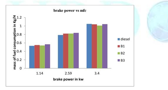
Graph 1: mass of fuel consumption Vs brake power of a diesel and its blends
