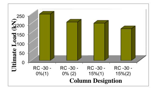
Figure 3.Compressive strength of all columns with M30 grade-comparision
