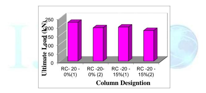
Figure 2.Compressive strength of all columns with M20 grade-comparision
