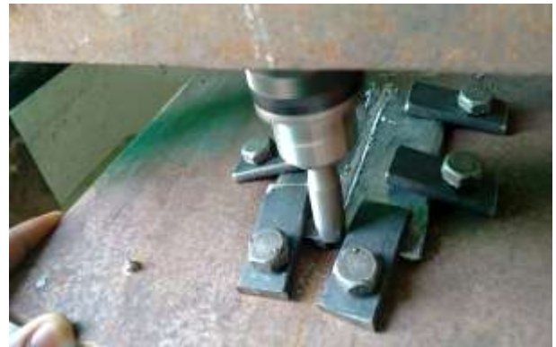
Fig. 10 End of FSW Process
