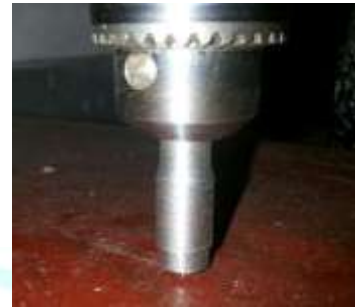
Fig. 6 Fabricated MS tool fitted on drill chuck of the setup
