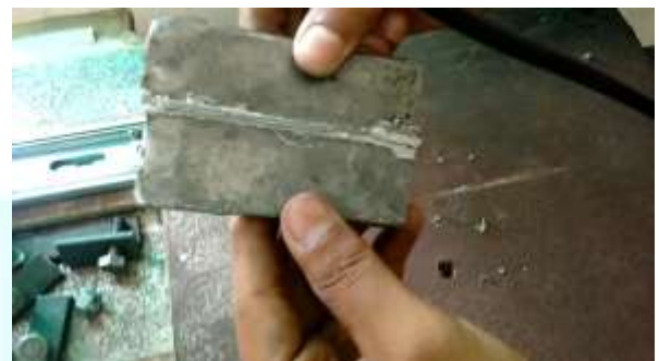
Fig. 11 Successful Joining of Lead alloy Plates
