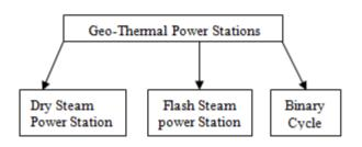
Fig 5. Classifications of geothermal power stations [2]
