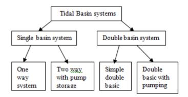
Fig 3. Classification of tidal basin constructions
