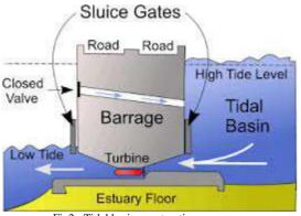
Fig2: Tidal basin constructions
