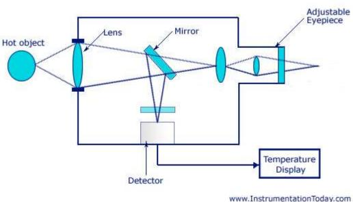
Block Diagram of Radiation Pyrometer
