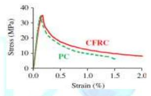
Fig: 2 Stress v/s strain graph for CFRC & PC. (Source: Google)
