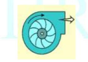
Fig.1. Backward curved centrifugal blower
