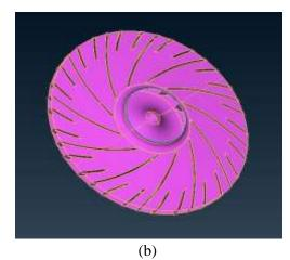
**Fig.5.** (a) Splitter at middle of the blade (b) Two Splitters per blade
