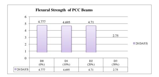
Fig. 6. Flexural Strength of Concrete Beams at 28 days
