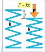
Figure 3. spring mechanics
