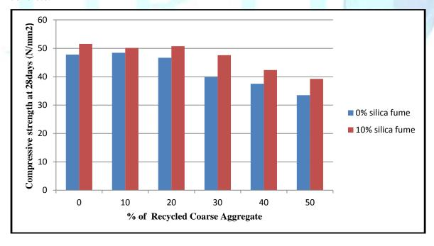
**Figure 4:** Effect of recycled coarse aggregate on compressive strength of concrete at 28days
