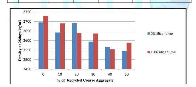
Figure 1: Effect of recycled coarse aggregate and silica fume on density of concrete
