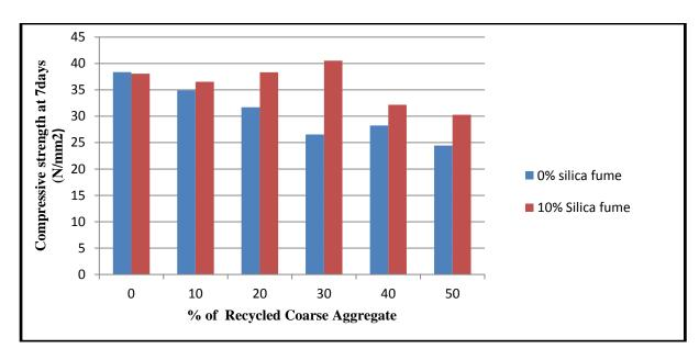
**Figure 3:** Effect of recycled coarse aggregate on compressive strength of concrete at 7days
