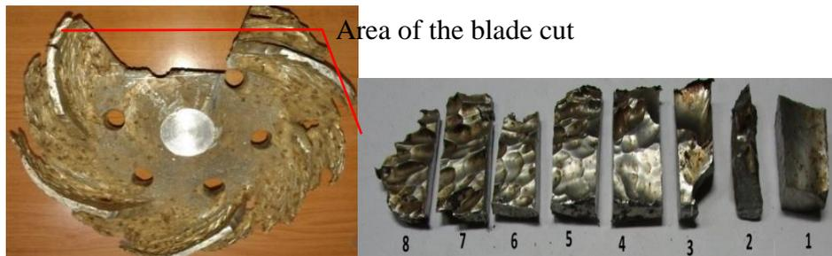
Figure 1. Cut made to a blade of selected samples.
