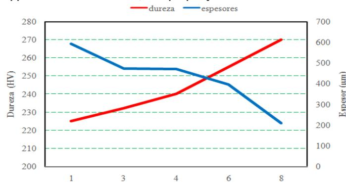
Figure 8. Hardness vs. thickness behavior.
