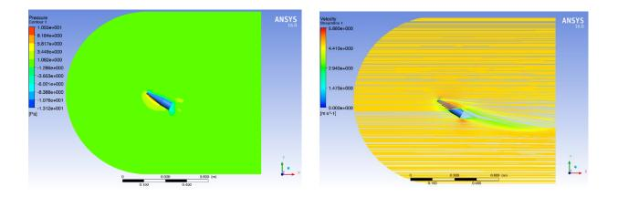
Figure 13 : The pressure and velocity contour for 57 mm projectile at 45°AOA
