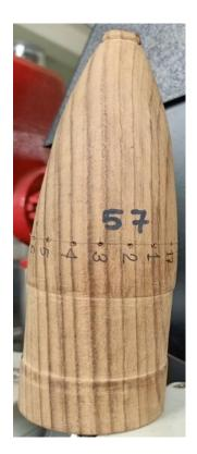
Figure 1 : Dummy Model of existing 37 mm & 57 mm Projectile
