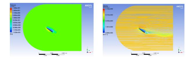
Figure 12 : The pressure and velocity contour for 37 mm projectile at 45°AOA
