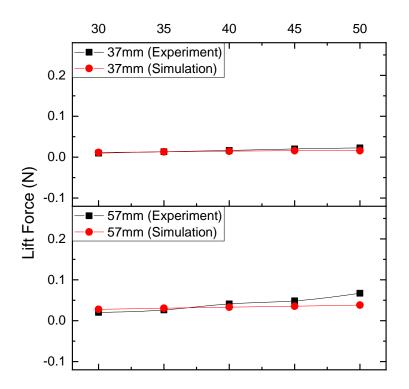
Angle of Attack (Degree) Figure 9 : Angle of Attack vs Lift Force.
