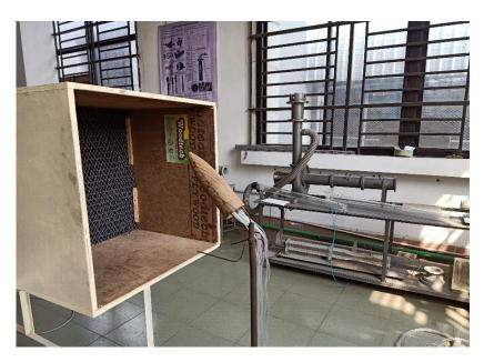
Figure 4: Experimental setup of projectile for measuring static pressure.
