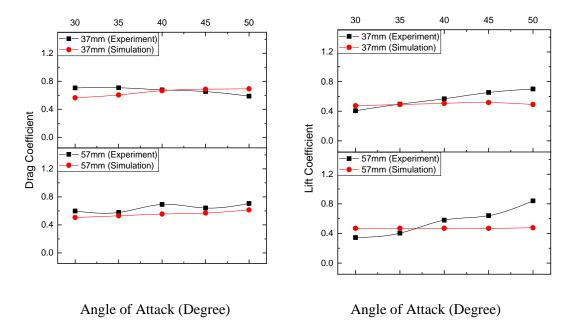
Figure 10 : Angle of Attack vs Drag and Lift Coefficients.
