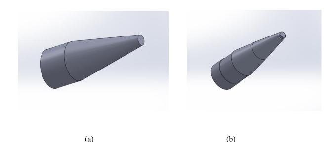
Figure 5. Geometry files for CFD simulation of (a) 37 mm and (b) 57 mm Projectiles
