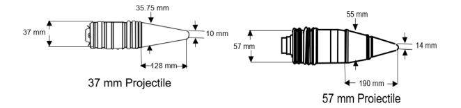
Figure 2 : Dimensions shown in Dummy Projectiles
