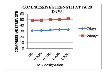
Figure No. 5: Graph comparing compressive Strength for 7 and 28 days
