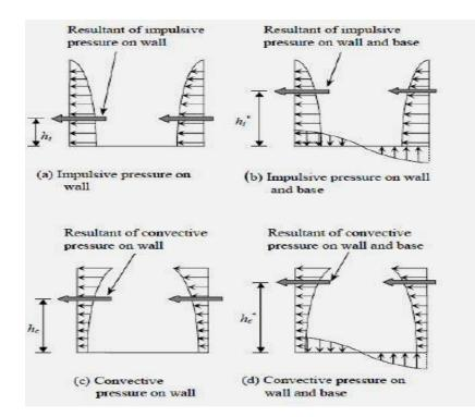
The above figure depicts the hydrodynamic pressure distribution for both the cases and their corresponding centre of pressures where as the  $h_i^*$  and  $h_c^*$  are the height of pressure inclusive of base pressure (Sloshing effect).
