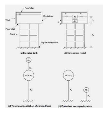
The total mass of water is divided into two different masses as illustrated in the above figure the mass of water which moves along with the tank wall with the horizontal excitation is known as Impulsive Mass ( $m_i$ ) and on the other hand the mass of water which moves relative to the tank wall is known as Convective Mass whereas the  $K_s$  and  $K_c$  are the corresponding stiffness of the structure and the convective mass of water.
