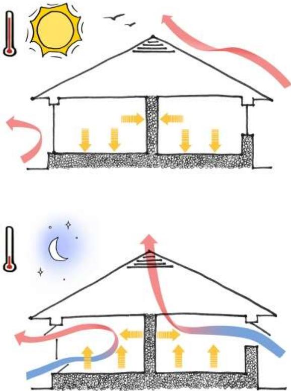
**Fig. 6** difference between day and night ventilation
