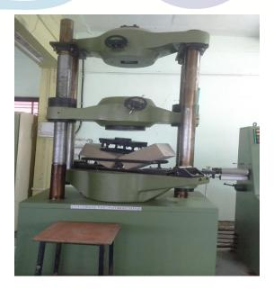
Testing Of Concrete Beam Specimen
