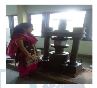
Testing of Concrete Cube Specimen
