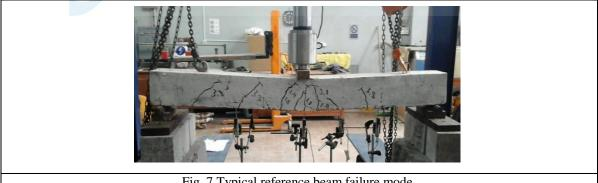
Fig. 7 Typical reference beam failure mode
