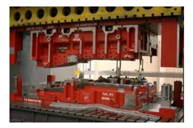
Fig 2 A STAMPING MACHINE SHOWING THE UPPER AND LOWER DIES(Allen Bradley)
