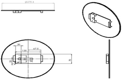
Fig 11: Dimensions of the latch shield.
