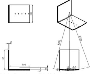
Fig 8: Dimensions of the limb mechanism.
