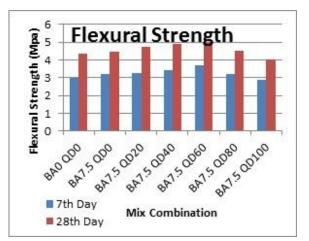
Figure 4.9 Flexural Strength Test values
