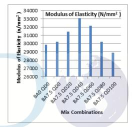
TABLE 4.8 DENSITY AND MODULUS OF ELASTICITY ALL CONCRETE MIXES
