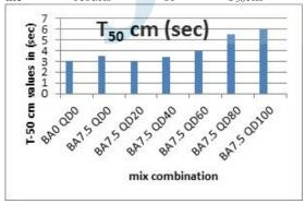
Figure 4.2 T<sub>50</sub> cm Slump Test Values
