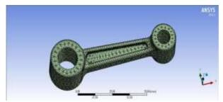
Fig.4. Meshed model of connecting rod
