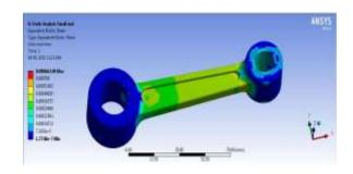
Fig.13.Al6061- Von mises strain
