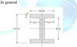
Fig.2. Standard dimensions of I section
