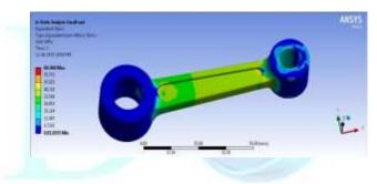
Fig.14. Al6061+B4C - von mises stress
