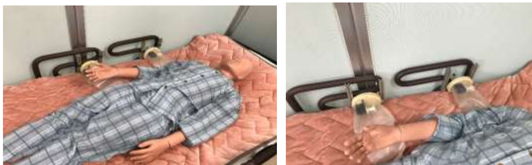
Figure 9. Installation of Soft Robot-arm on the handrail of the bed.
