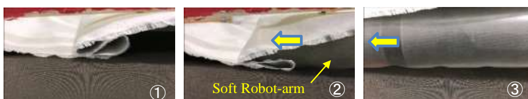
Figure 5. State where wrinkles of clothes are removed by Soft Robot-arm.
