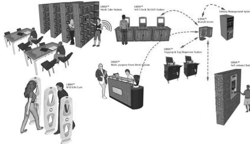
The RFID reader sends out electromagnetic waves and the tag antenna is enabled to receive these waves. “When the tag antenna enters the RF (radio frequency) field, the tag’s microchip circuits are powered by signals from this RF field created by the reader. The chip then modulates the waves and the tag sends them back to the reader. The reader converts the signals received from the tag into digital data and sends it to a computer.”
