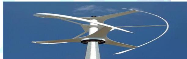
Fig:- 1 vertical axis wind turbine
