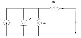
Fig-3 Equivalent circuit of a solar cell
