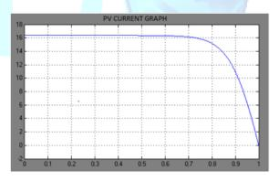
FIGURE 7 I-V CHARACTERISTICS OF PV ARRAY WITH CONSTANT TEMPERATURE AND IRRADIANCE
