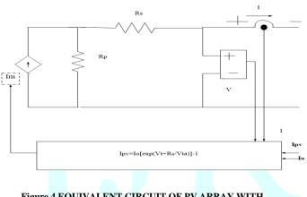
Figure 4 EQUIVALENT CIRCUIT OF PV ARRAY WITH CURRENT EQUATION
