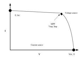
Figure 5 CHARACTERISTICS I-V CURVE OF A PRACTICAL PV DEVICE
