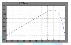
FIG 6 P-V CHARACTERISTICS OF PV ARRAY WITH CONSTANT IRRADIANCE AND TEMPERATURE
