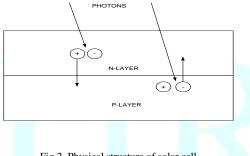
Fig 2. Physical structure of solar cell
