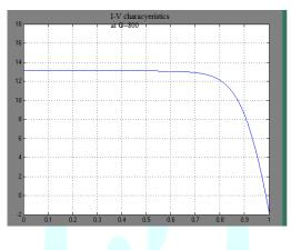
Fig 9 I-V characteristics with G=800kW/m^2
