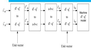
Fig -3 Vector Control principle
