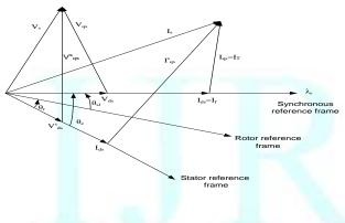
Fig -4 Phasor diagram of Induction machine
