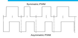
Fig 1 – Different types of PWM signals
