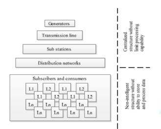
Fig 4(a).Shows Block Diagram of Conventional Grid
