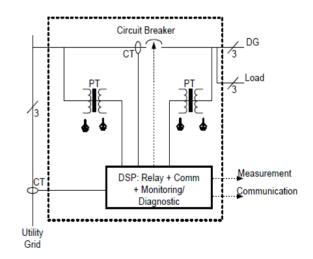
Fig.3 shows schematic diagram of circuit breaker on connection to the grid
