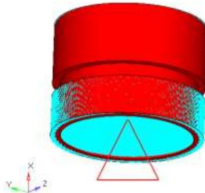
Fig-5.6: Boundary conditions applied on the bearing cup
