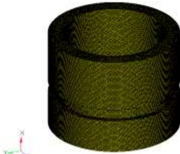
Fig-5.3: 2D Meshing of Bearing cup
