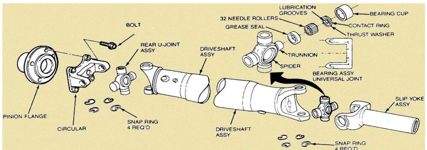
Fig-1.1. Bearing Cup Assembly with drive shaft
