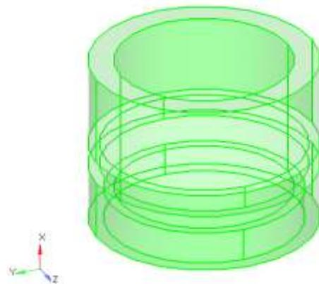
**Fig-5.2:** Bearing cup Surface refining for 2D meshing
