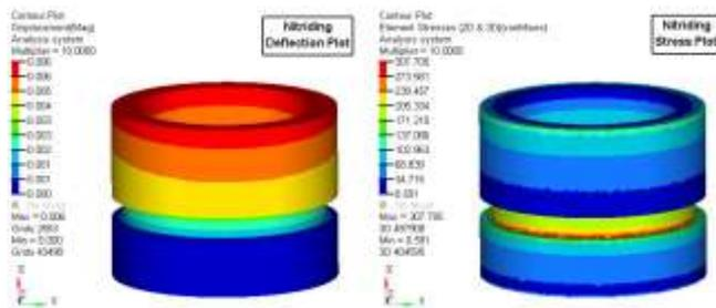
**Fig-5.10:** Deflection and Stress Plot (Cup without Nitriding)
