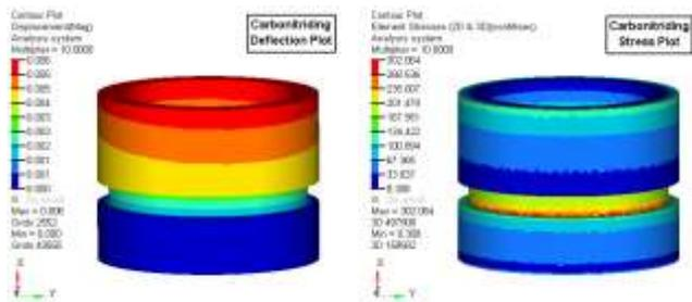
**Fig-5.9:** Deflection and Stress Plot (Cup without Carbonitriding)
