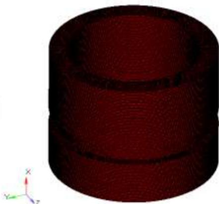
Fig-5.4: Meshed model of Bearing cup
