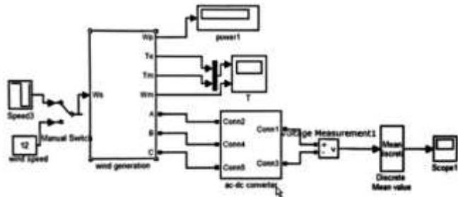
Fig 1.1.1., Wind energy system model
