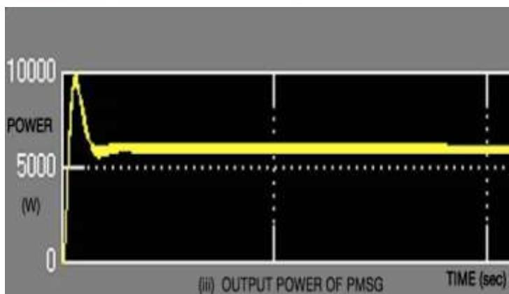
Fig 3.3., Output Power of PMSG
