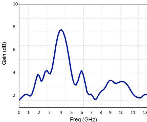
**Figure 7.** Proposed dual band antenna gain
