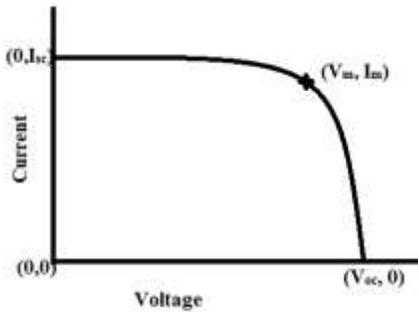
Fig 2: V-I characteristics of solar cell
