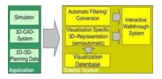
Fig.4. Process of image generation.
