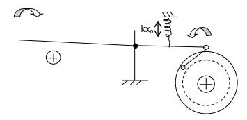
Figure 6: Cam slides off the lever, forcing the spring to return to suddenly to original X<sub>0</sub> from extended X<sub>2</sub>
