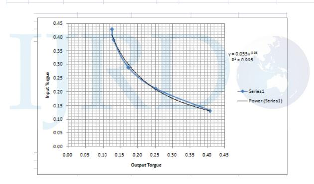
Figure 4: Graph characterizing input/output torques in Figure 1 tests
