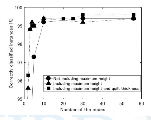
Fig. 8. The percentage of correctly classified instances for datasets including both thin and thick quilts depending on the number of nodes.
