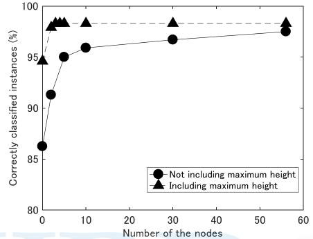
Fig. 5. The percentage of states correctly classified for a thin quilt depending on the number of sigmoid nodes.
