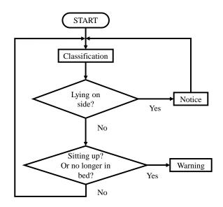
Fig. 1. Flowchart of the awakening detection system.
