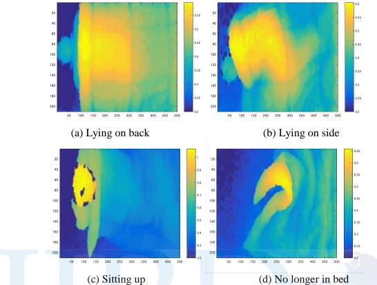
Fig. 6. Examples of height data for the four cases. The subject is covered by a thick quilt. One pixel is equal to 4.5 mm, and the color bars are in meters.
