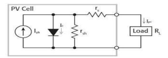
Fig:1 Equivalent circuit of PV cell: one diode (<u>https://www.researchgate.net/figure/284810777\_fig 2Single-diode-equivalent-circuit-model-of-solar-cell.</u>)
