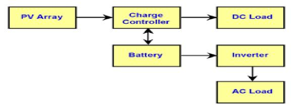
Fig:4 Block diagram of PV system. (http://www.fsec.ucf.edu/en/consumer/solar\_electricity/basics/types\_of\_pv.htm.)
