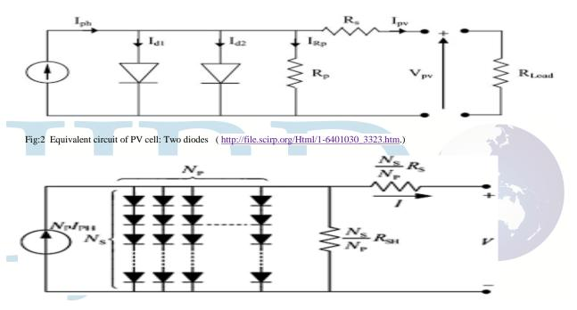
Fig:3 Equivalent circuit of PV cell: Multiple diodes ( http://link.springer.com/content/pdf/10.1186%2Fs40068-015-0047-9.pdf.)
