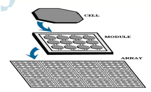
Fig:6 Solar Cells/Modules (http://www.globalspec.com/learnmore/optics\_optical\_components/optoelectronics/photovoltaic\_cells.
