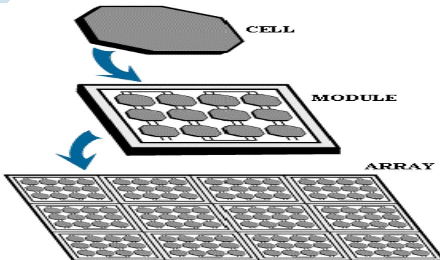
Fig:6 Solar Cells/Modules ([http://www.globalspec.com/learnmore/optics\\_optical\\_components/optoelectronics/photovoltaic\\_cells](http://www.globalspec.com/learnmore/optics_optical_components/optoelectronics/photovoltaic_cells)).
