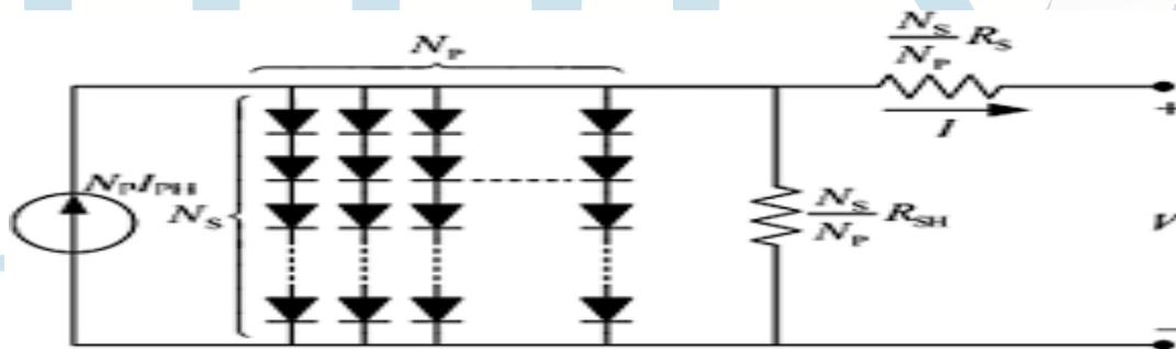
Fig:3 Equivalent circuit of PV cell: Multiple diodes (<http://link.springer.com/content/pdf/10.1186%2Fs40068-015-0047-9.pdf>.)
