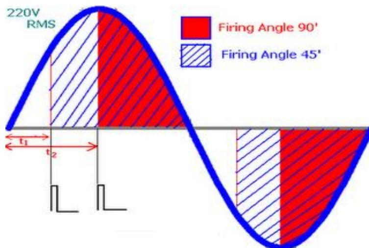
**Fig.3 Representation of firing Angle of TRIAC**
