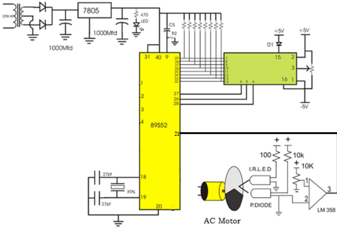
Fig. 5 Circuit of Speed measurement
