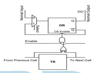
Fig 3. Selective triggering architecture
