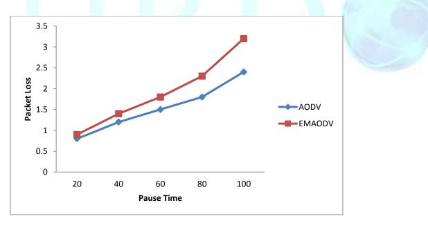
Figure 2: packet loss vs. pause time of AODV & EMAODV
