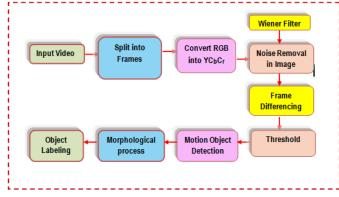
Fig.1 Flow chart for the proposed Algorithm
