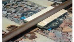
Fig5. Axial counter on track with transmitter and receiver connected via fibre optical cables.
