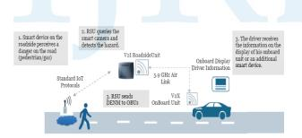
Fig1. IOT sensors and smart devices will allow a seamless integration of V2X technologies with smart cities that will increase road safety. For instance, vehicle and roadside sensors will be able to detect road hazards and pedestrians in the road and the onboard unit will alert the driver to take evasive action.
