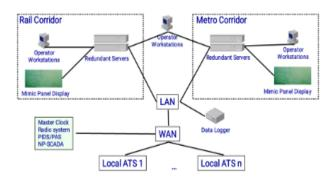
Fig8. Networking system of trains with the local ATS and redundant servers.
