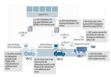
Fig2. V2X integration with smart city systems will improve freight management. For example, a truck's cargo can inform its environment about potentially dangerous goods, either by direct communication, or optionally via a central ITS station.
