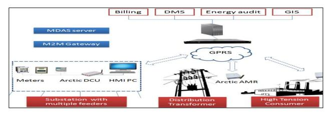
Fig. 1. Architecture of MDAS system
