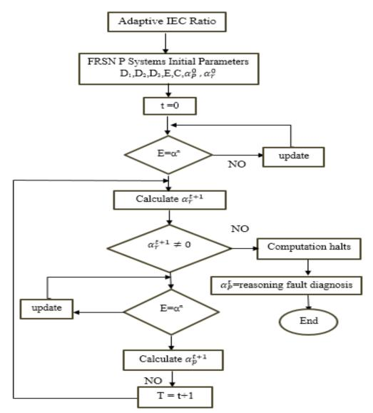
Figure 3. FRSN P systems transformer fault diagnosis flow chart.
