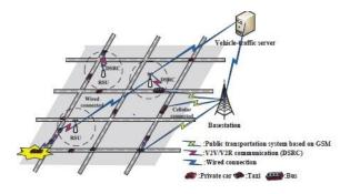
Figure 2: Hybrid VANET-enhanced network architecture
