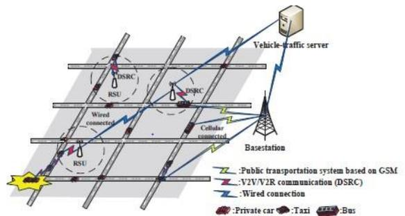
Figure 2: Hybrid VANET-enhanced network architecture
