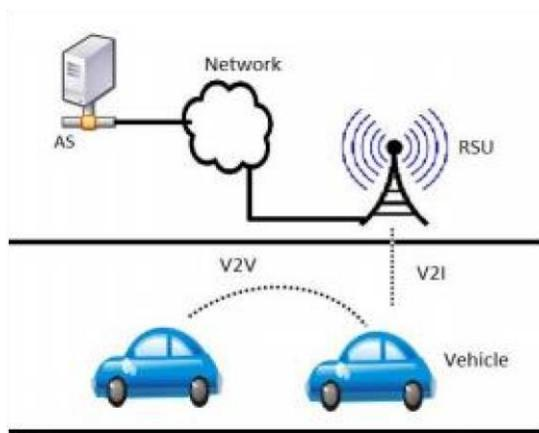
Figure 1: V2V and V2I communication
