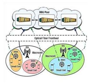
Figure 6: Cloud Radio Access Network Architecture
