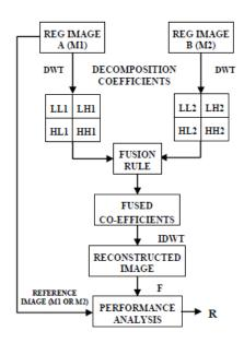
Fig 1: Flowchart of DWT Algorithm
