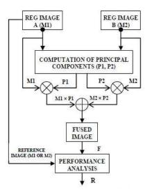
Fig 2: Flowchart of PCA Algorithm
