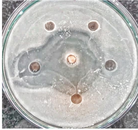
Figure 7. An inhibition zone around the wells filled with AgNPs (No inhibition zone around the untreated wells)
