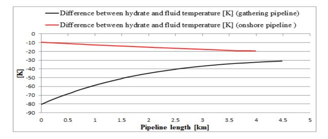
Figure 5. Difference between hydrate and fluid temperature in the onshore and gathering pipeline.
