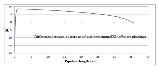
Figure 4. Difference between hydrate and fluid temperature in the offshore pipeline.
