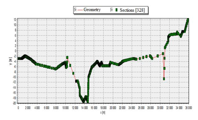
Figure 2.Geometry of the offshore pipeline generated by OLGA software.
