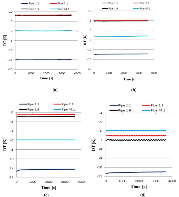
Figure 7. Difference between hydrate and fluid temperature (DT) in the different pipe section of the offshore pipeline with: (a) 0% MEG, (b) 10% MEG, (c) 20% MEG (d) 40% MEG.
